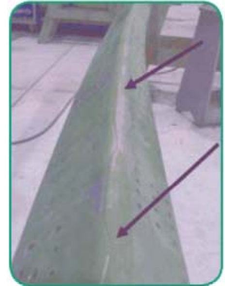
Arrows indicate crack in attach angle
